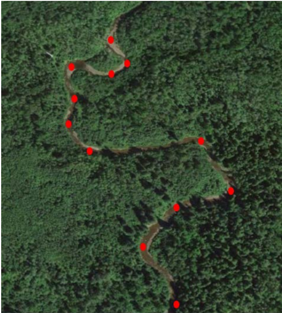
Figure A.8. Points identifying the stream channel at farthest landward point of each meander bend
